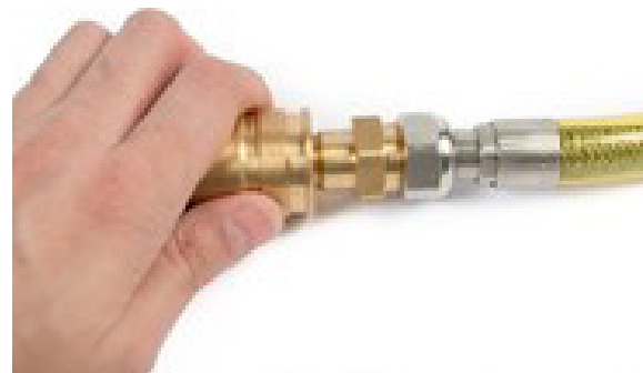
Reconnect by pushing the nipple into the female end.
